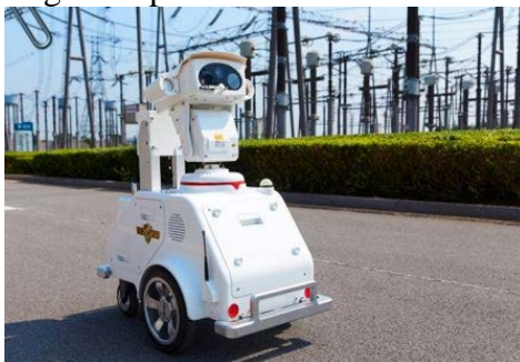
Figure 1 Substation Patrol Robot
